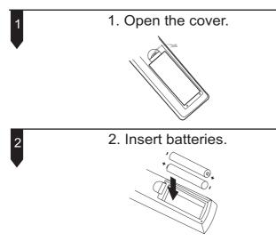
Make sure to match the "+" and "-" of the batteries with the marks inside the battery compartment.
